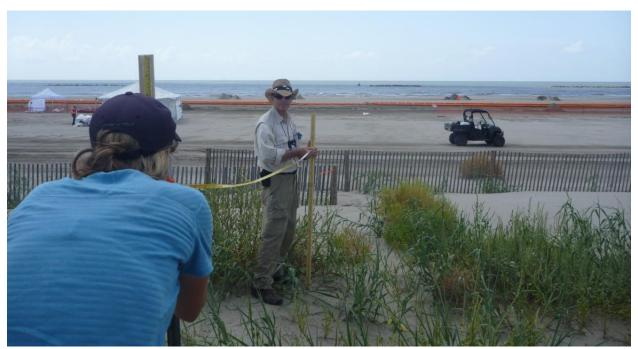
Figure 1. Beach profiling using the rod-and-horizon method.
