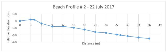
Figure 2. Example of beach profile: note the intermediate measurement points at 4 m and 28 m along the transect
