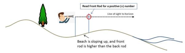
This number is the POSITIVE height difference of the slope of the beach between the two rods.
