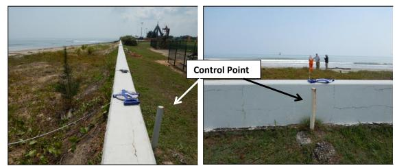
Figure 9. Example of a permanent control point
